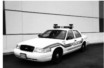
This B.C. traffic enforcement vehicle has four ALPR cameras mounted on the light bar. Infrared illuminators allow the cameras to operate in any light or weather conditions.
