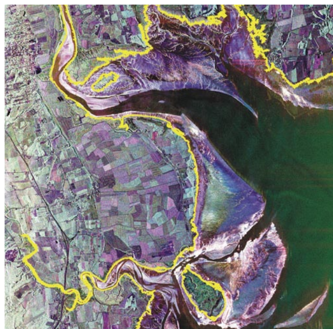
In this CV-580 C/X-SAR multi-polarization composite image of the Minas Basin, Nova Scotia, acquired during low tide conditions, the colourful patterns indicate differences in the information content of the three images. The yellow line marks the boundary between dry land and tidal plane. Oceans and coastal applications benefit from the versatility of RADARSAT-2. (Image CCRS, 1999)
