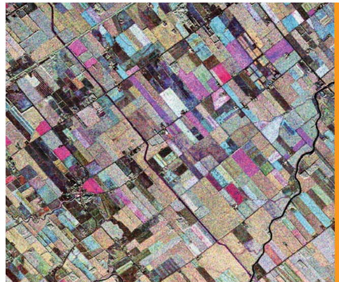
Agricultural fields south of Ottawa in a composite C/X-SAR multi-polarization image. Diversity of polarization, incidence angles, and spatial resolutions offered by RADARSAT-2 provide valuable information for agricultural management such as crop identification, soil conservation methods, and soil moisture. (Image: CCRS, 1998)
