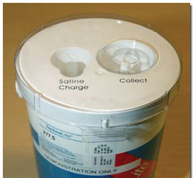
Figure 15. Top view of Tc-99m generator in Figure 14. Note: The holes would contain sharp needles to accommodate vials.
