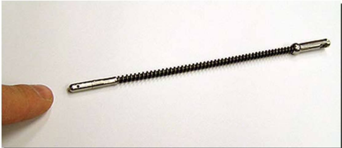
Figure 37. Standard source used inside an exposure device. The radioactive source would be in the tip of the device, near the finger in the photograph. If you see a source like this, do not touch it and immediately back up 400 m and refer to Table 1 in Appendix A to determine the gamma dose rate.
