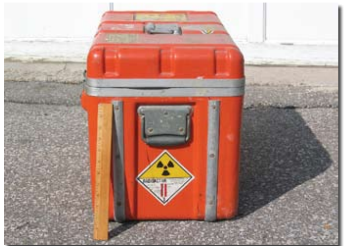
Figure 10. Campbell Pacific Nuclear series portable nuclear gauge in shipping container with a Category-II Yellow label.
