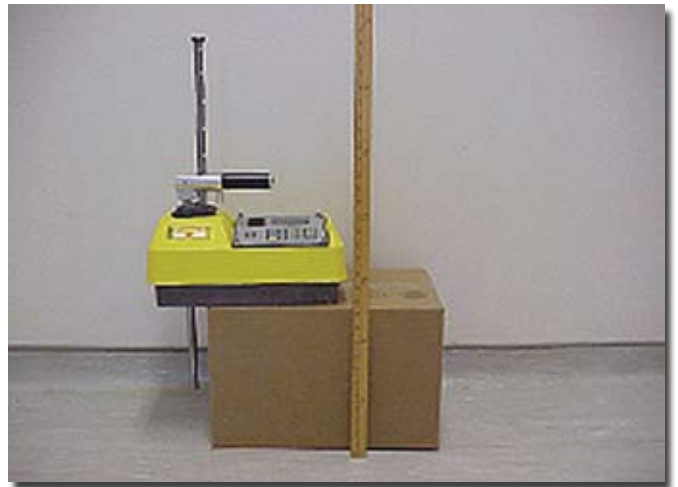
Figure 8. Troxler series portable nuclear gauge with source rod extended
