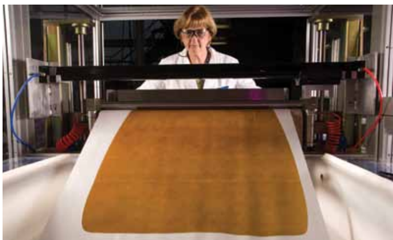
NRC technical officer Linda Layton casts a sheet of a novel polymeric membrane material for gas permeability testing at NRC-ICPET.
