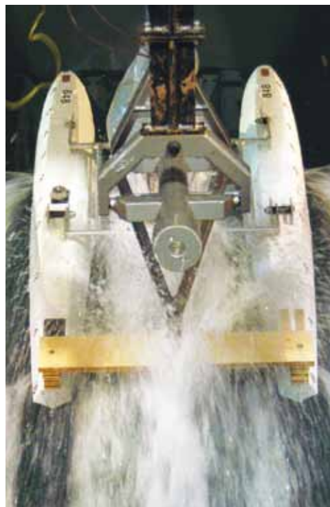
A model seaplane float is tested at the NRC Institute for Ocean Technology’s towing tank facility in St. John’s.
