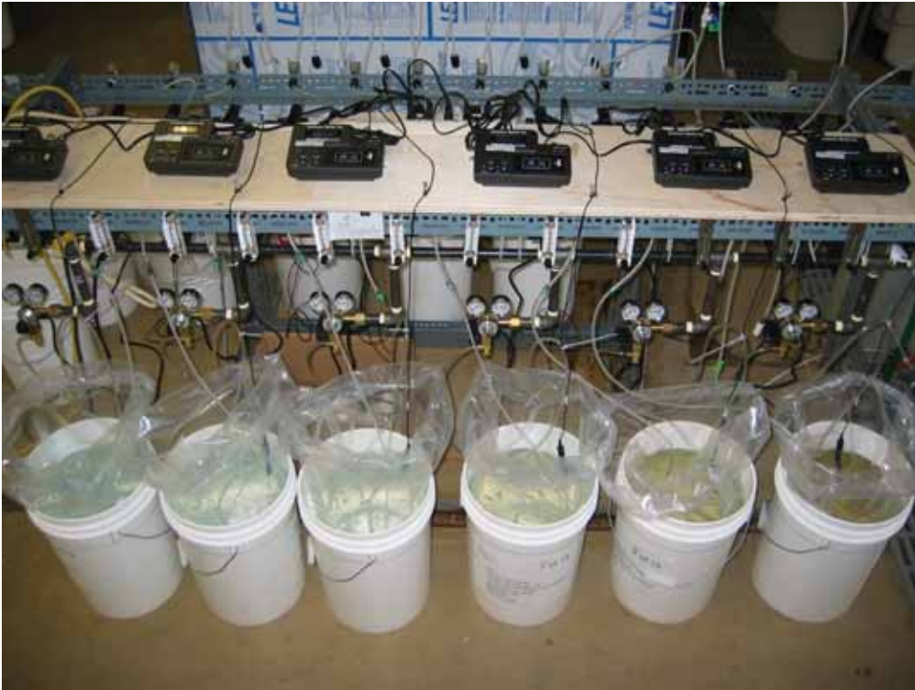
Figure 11 Overview of Setup for LC50 Test Using pH Controller Technique
