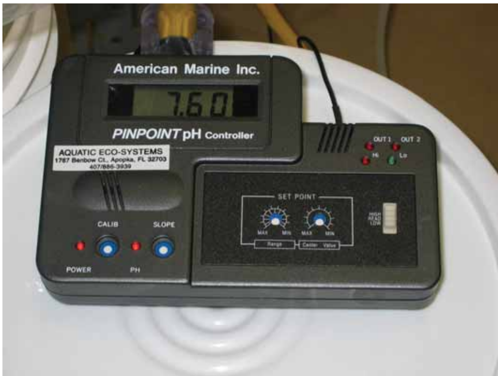
Figure 12 Example of pH Controller Unit
