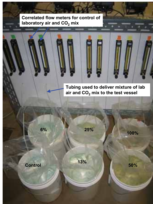
Figure 5 Plastic Pails Used for CO 2 Injection Technique
