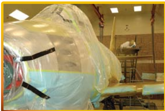
Corporal Mike Williams (above left), and Corporal Jeff Brawn (above right) spray a layer of gold aerospace paint onto the surface of the Korean War vintage Sabre Mark 5/6 aircraft. CF Photos by Pvt P. Turney
