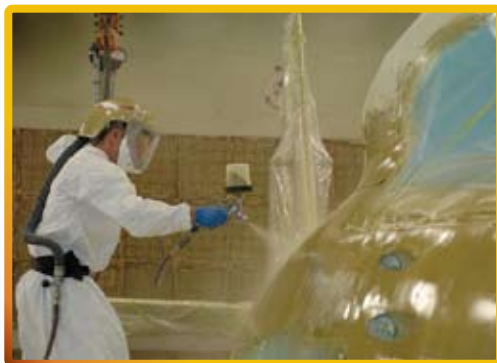
Corporal Mike Williams (above left), and Corporal Jeff Brawn (above right) spray a layer of gold aerospace paint onto the surface of the Korean War vintage Sabre Mark 5/6 aircraft. CF Photos by Pvt P. Turney
