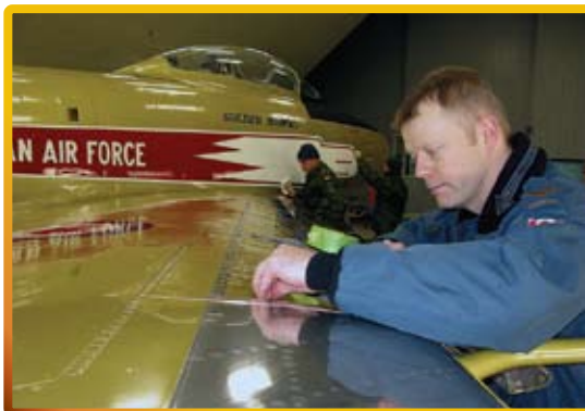
Corporal Mike Williams (above left), and Corporal Jeff Brawn (above right) spray a layer of gold aerospace paint onto the surface of the Korean War vintage Sabre Mark 5/6 aircraft. CF Photos by Pvt P. Turney
