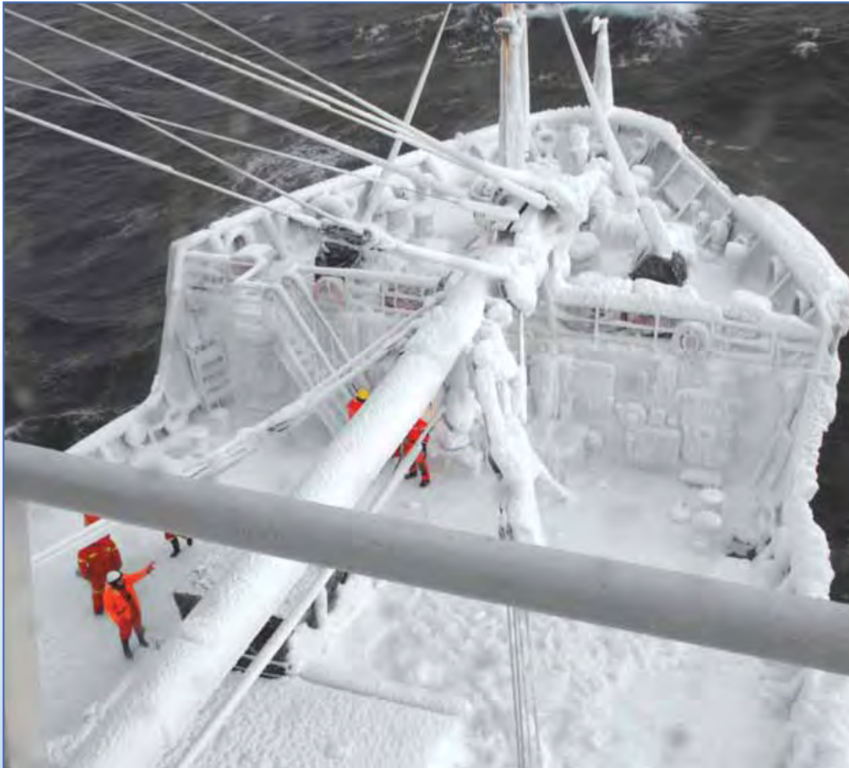
Ice Accumulation on the CCGS George R. Pearkes - High-endurance Multi-tasked Vessel/Light Icebreaker
