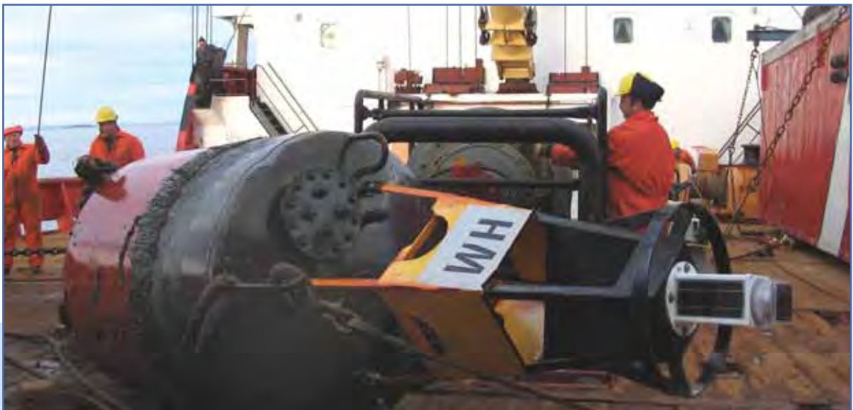
CCGS Ann Harvey, High-Endurance Multi-tasked Vessel/Light Icebreaker doing buoy work
