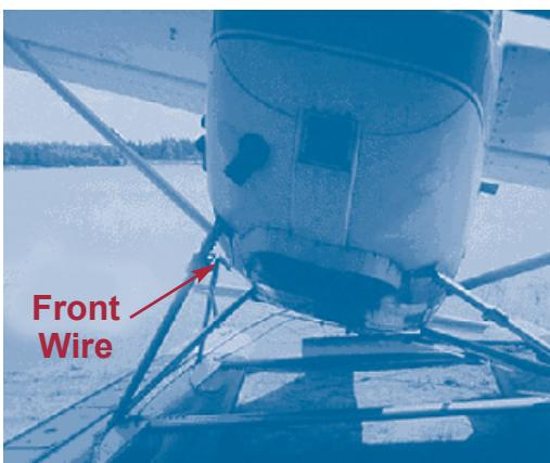
with the water. This caused the aircraft to veer left abruptly, displacing a considerable amount of water, but I managed to keep the aircraft from inverting. This caused all the fittings on the float struts to fail. The final resting position of the aircraft was engine pointing up, tail and left wing partially submerged. The aircraft was towed back to my property where it was beached. Upon inspection it was found that both cross wires were broken (left lower to right upper side)."
