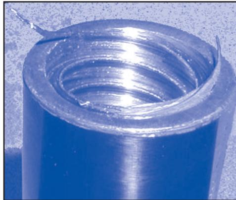
*The submitter added that the overhaul facility had disassembled the actuator and discovered excessive wear and stripped threads on the nut, with scoring on the screw threads. The unit is being sent to Raytheon for further analysis.*
