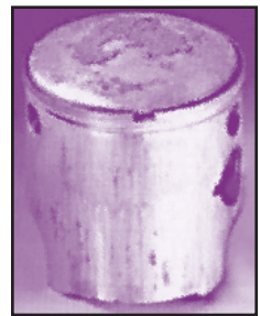
Piston deterioration caused by detonation
