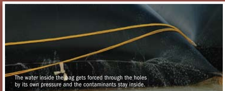
The Geotubes treated 80,000 cubic metres of water at Tundra Mine this summer. That's more than the volume of 30 Olympic-sized swimming pools!
