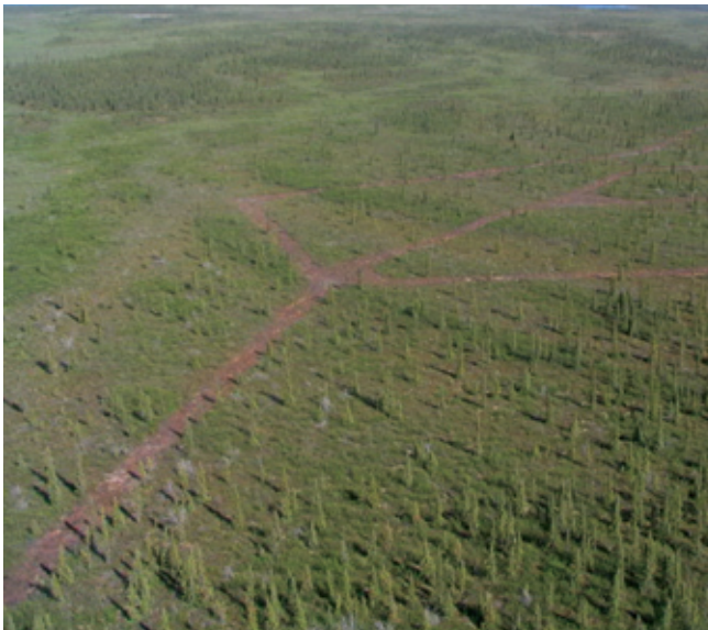
FIGURE 2. Determine if existing roads can be used. Proper planning may have prevented the network of roads shown in this photograph.
