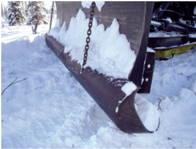
FIGURE 28. A smear blade raises the bulldozer blade off the ground surface.
