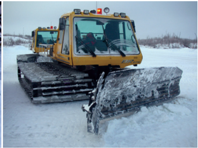
FIGURE 29. A low ground pressure vehicle, such as a snowcat, can be used for a first pass to compact snow on a winter road.
