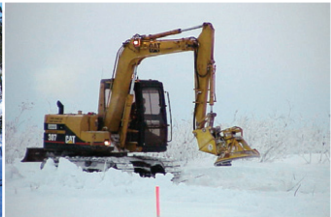
FIGURE 12. A brush cutter can be used to cut and dispose of brush.
