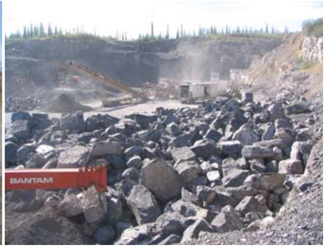
FIGURE 23. Excessive dust caused by crushing operations can be mitigated by spraying water or using dust skirts on conveyors.
