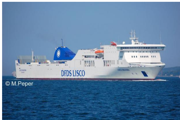
Figure 5-4: M.F. Lisco Maxima, 2009-built, 600 passengers, 500+ autos
