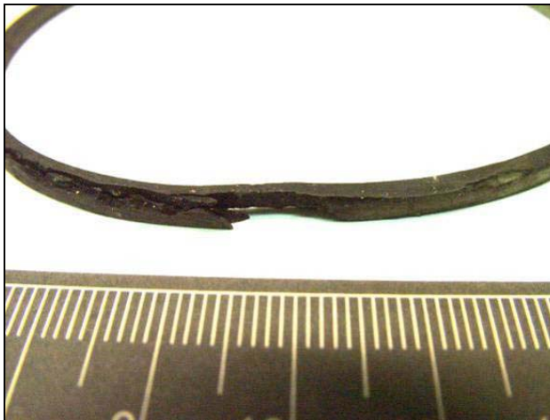
Photo 3. Damaged O-ring gasket
