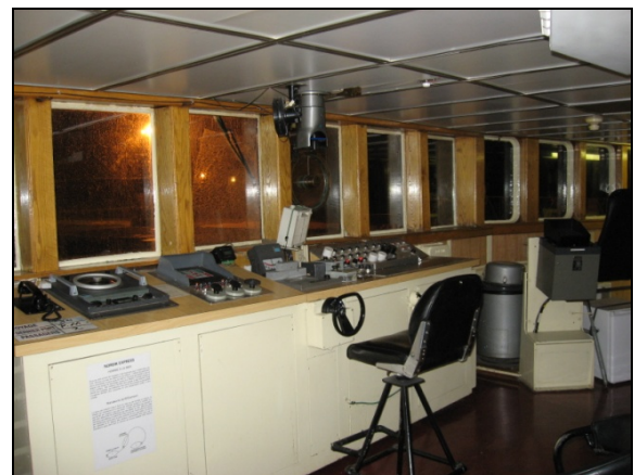
Photo 2. Bridge centre console showing the starboard radar. The other radars and ECS are out of view to the left (port).
