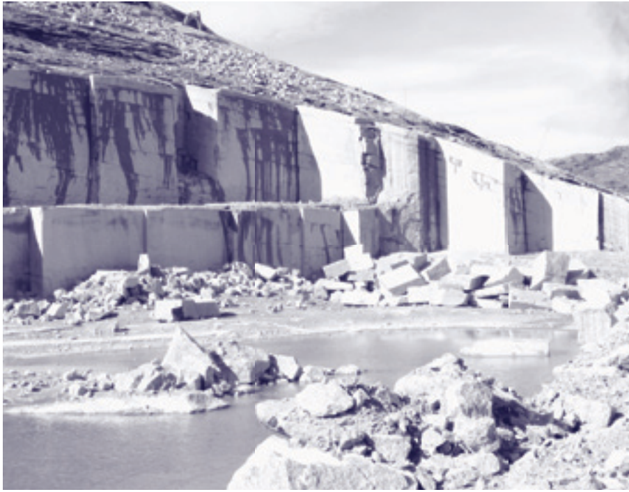
The Labrador Inuit Association's Labradorite quarry at Ten Mile Bay. Blocks weighing from 10 to 30 tonnes are shipped to Italy where they are sold to customers from around the world. Source: Labrador Inuit Development Corporation.
