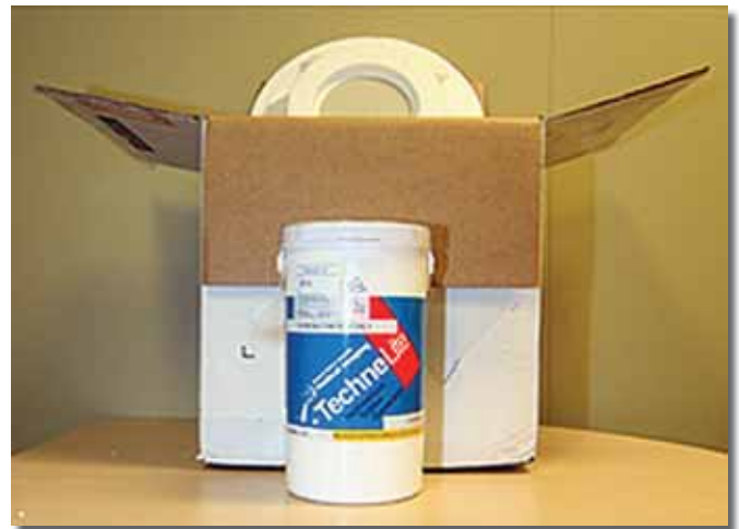
Figure 14. Tc-99m generator as seen after removing styrofoam shown in Figure 13 (note height of about 25 cm).
