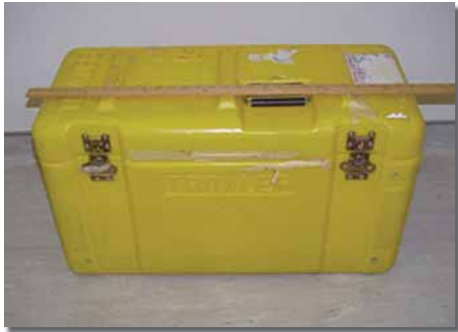
Figure 5. Type A package that contains a Troxler series portable nuclear gauge.
