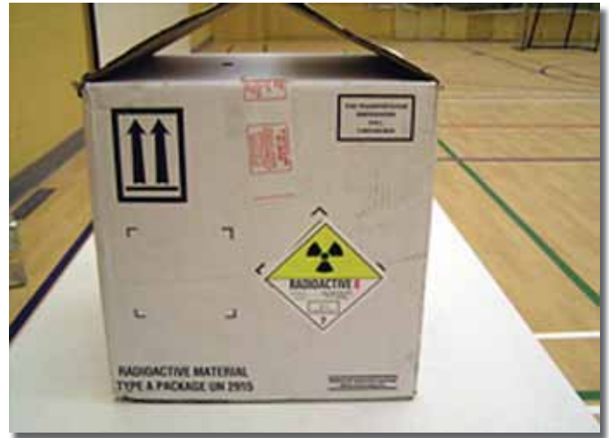
Figure 13. Box containing a technetium (Tc-99m) generator.
