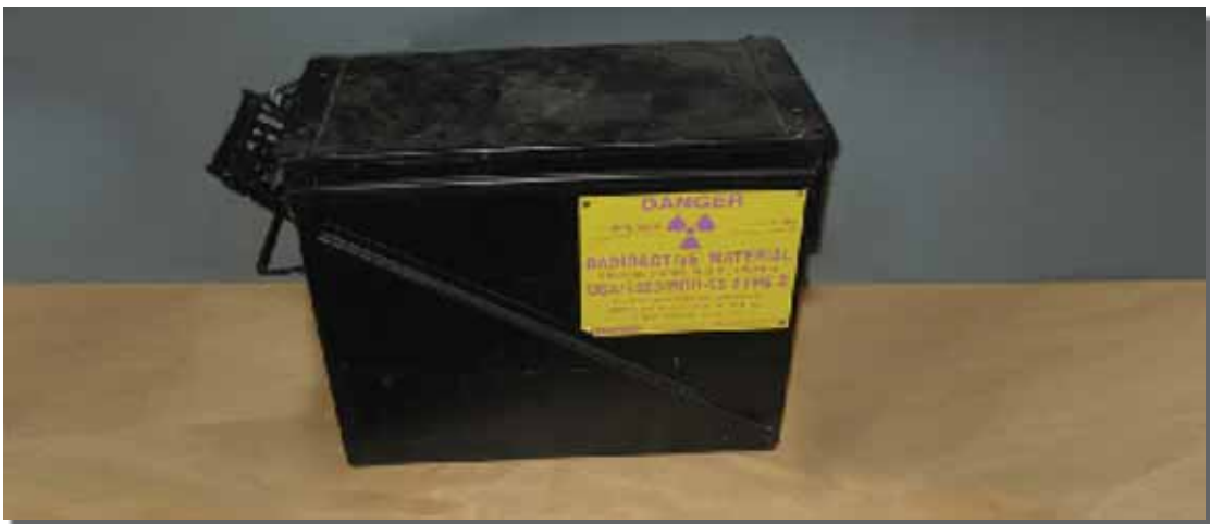
Figure 31. Side view of container shown in Figure 30. Note: This particular package does not require a category label , but has a yellow warning label that declares the radioactive contents.
