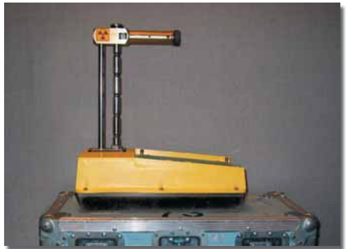
Figure 9. Humboldt series nuclear gauge with source rod gauge with source rod in the fully shielded position.
