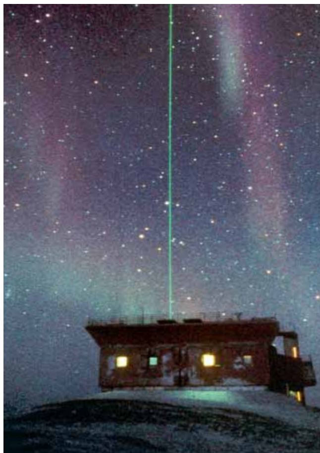
Figure 20. The Eureka Polar Environment Atmospheric Research Laboratory on Ellesmere Island in the Canadian high Arctic. The beam from the top of the roof is the LIDAR laser.
