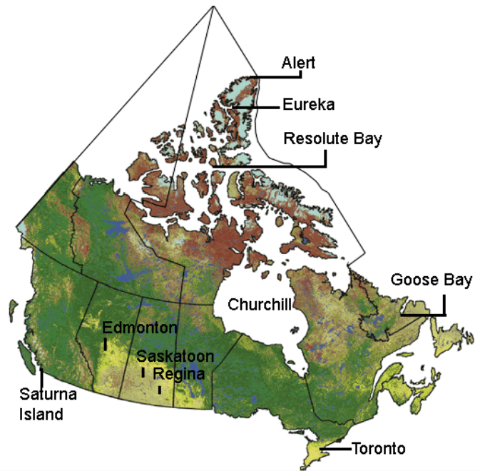
Figure 16. The Canadian ozone observation network consists of 10 Brewer spectrophotometers. In southern Canada, they are located Goose Bay (Labrador), Toronto, Churchill (Manitoba), Regina, Saskatoon and Edmonton, and on Saturna Island in British Columbia. In the Arctic, Brewer instruments are located in Nunavut, at Resolute Bay, Eureka and Alert.
