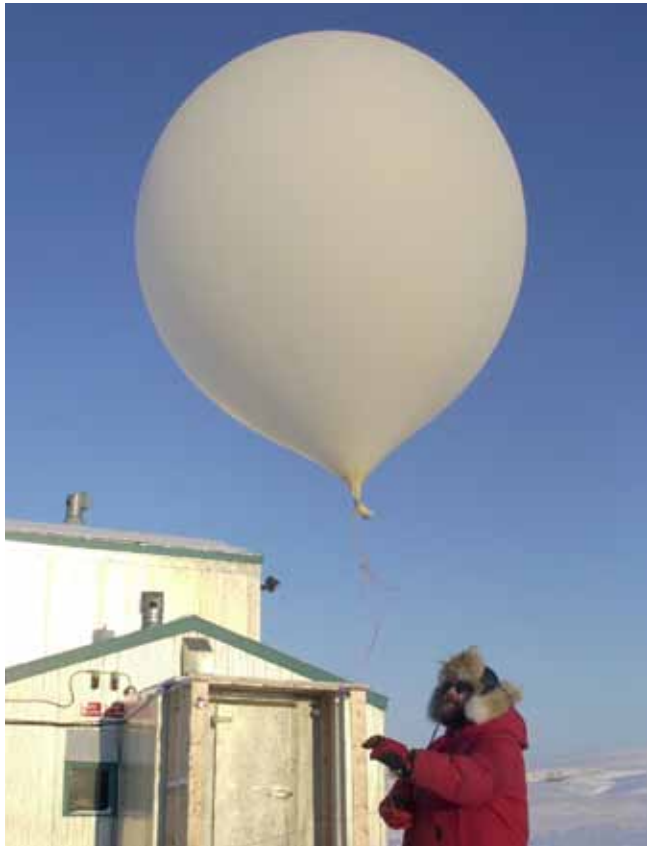
Figure 17. Canadian ozonesondes, such as the one shown on the left, are launched from Edmonton, Churchill, Goose Bay, Resolute Bay, Eureka, and Alert to provide ozone measurements at altitudes of up to 35 km.
