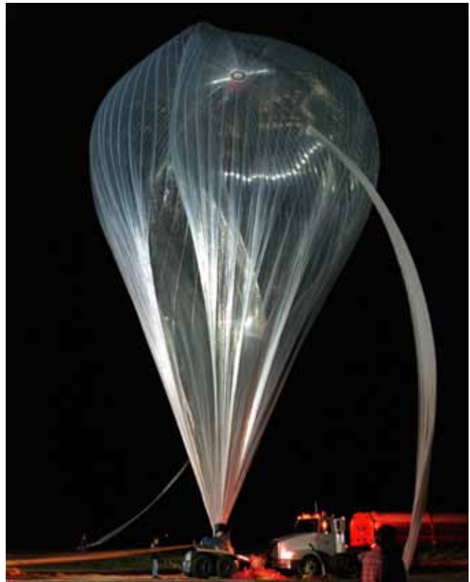
Figure 18. At ten storeys tall, the Mantra research balloon carries instruments in a small gondola to an altitude of 35 km.
