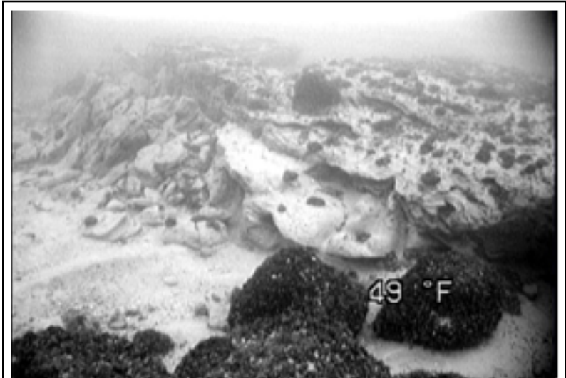
Figure 3. Underwater video image of cohesive clay ridge (light blocky material) surrounded by medium to coarse sand and large cobbles/small boulders.
