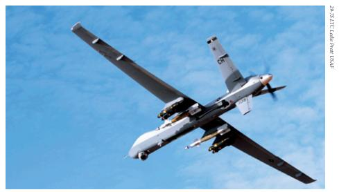
Figure 2: The payload of the MQ-9 Reaper varies based on the mission but often consists of GBU-12 laser guided bombs and AGM 114 Hellfire missiles
