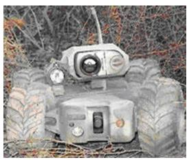
Figure 16: Dragon Runner with Mounted Camera (Note: This variant is not invertible.)<sup>42</sup>
