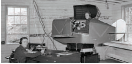
Link trainer, Royal Canadian Air Force Station. Canada. Department of National Defence / Library and Archives Canada / PA-136268
