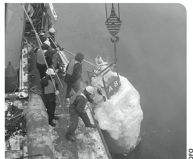
The crew of CCGS Tracy must remove the ice from the lifting rings on this lighted summer buoy before it can be brought aboard. It will be replaced by a winter spar (on the deck).
