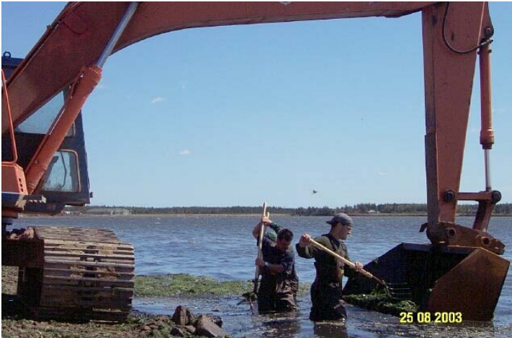
Figure A 2 : Algae harvesting from the platform built on the shoreline. On left, perforated excavator bucket; on right, modified trawl towed by the excavator (source: Coalition pour la viabilité de l'environnement de Shippagan et des Îles Lamèque et Miscou).
