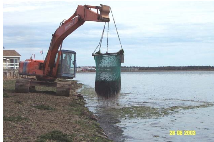
Figure A 2 : Algae harvesting from the platform built on the shoreline. On left, perforated excavator bucket; on right, modified trawl towed by the excavator (source: Coalition pour la viabilité de l'environnement de Shippagan et des Îles Lamèque et Miscou).
