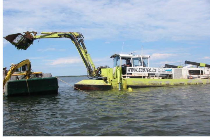
Figure A4: Algae harvesting in the bay (at sea) using an aquatic plant harvester (on left) and an amphibian excavator equipped with a modified perforated bucket (on right).
