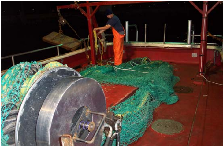
Figure A 3 : Algae harvesting in the bay (at sea) with modified traditional commercial fishing gear. On left, modified Devism trawl; on right, modified scallop dredge.
