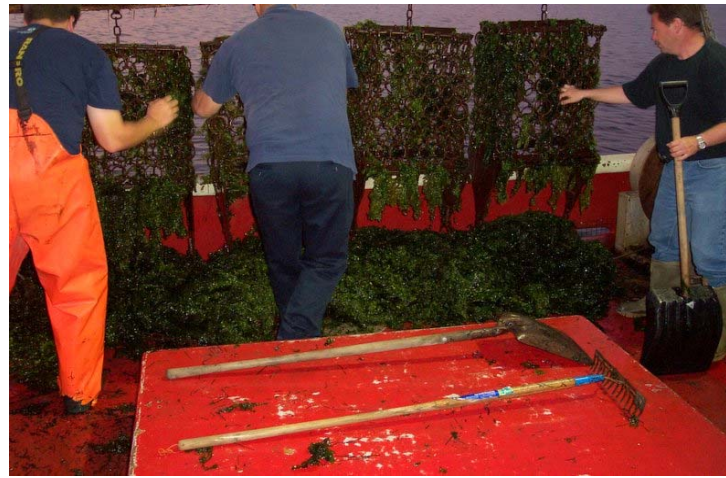
Figure A 3 : Algae harvesting in the bay (at sea) with modified traditional commercial fishing gear. On left, modified Devism trawl; on right, modified scallop dredge.
