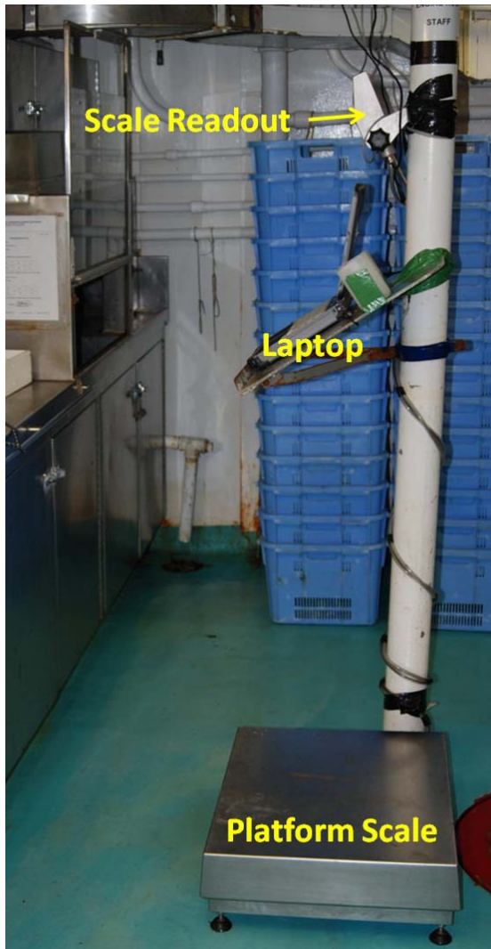
Figure 26. A typical Haul Card station setup.
