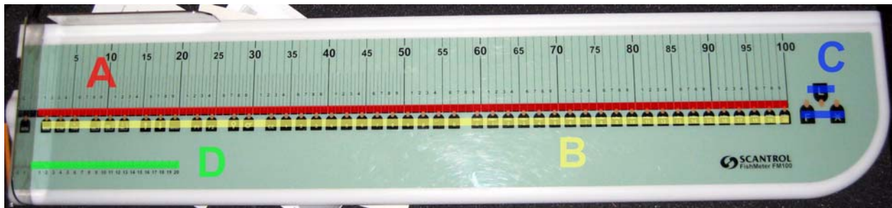
Figure 53. A 100 cm Scantrol FishMeter fish measuring board. A: Magnetic activation strip. B: Function keys. C: Mode selection keys. D: Millimeter measuring strip.
