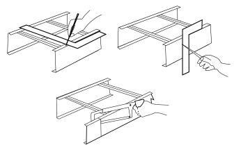
The next step is to drill holes for attaching the splice plate to the cut cable tray. To make sure the holes are in exactly the right place, Janet uses a splice plate bolted to a short piece of side rail punched with a standard hole pattern as a template. She lines up this template with the cut cable tray, marks the proper drilling location through the holes in the splice plate and drills the required holes in the cut cable tray.
