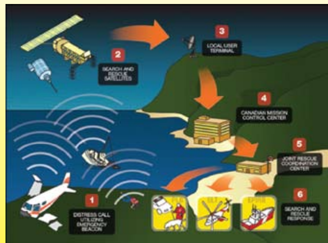
Fig. 1 – How the COSPAS-SARSAT system works.
