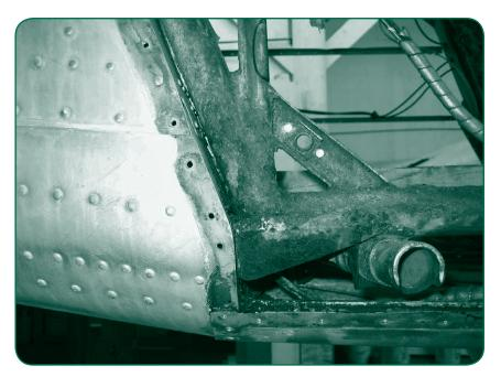
can allow water/moisture to enter the aircraft. In particular, the lower fuselage areas and any insulation blankets must be kept clean and dry. Additionally, ensure that all lower fuselage water drains are kept free to drain fluid overboard.
