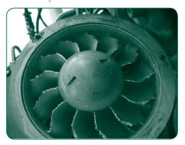
and become ingested into the engine. Aircraft had been subject to scheduled inspection less than 10 hours prior, with no defects noted at that time. Aluminum shavings from welded boss were found ejected out of the bleed valve and out of the exhaust. The steel union did not get ingested, but bounced around in the intake plenum causing substantial damage to the axial compressor.
