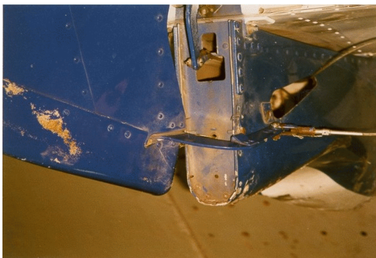
Figure 1 - Rudder jammed in 34-degree deflection
