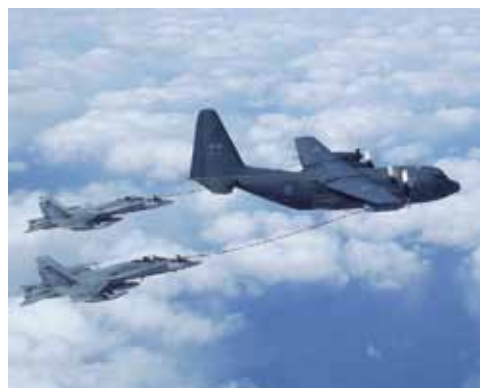
Figure 11. Two CF188 Hornets air refuel from a CC130T Hercules on a flight from Canada to Iceland to join Task Force Iceland at Keflavik Air Base, Iceland, in support of Op IGNITION. 45
