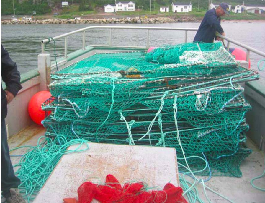
Figure 7. The cod pots were designed to fold flat to conserve deck space. Here 15 are shown stacked on the aft deck of a small fishing vessel.
