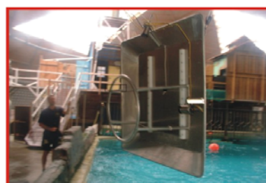
The plate with hoop, sliding door, hydrophone and 2 cameras
