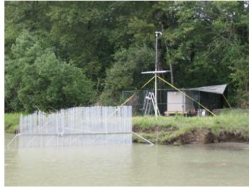
Fig. 4. The telescopic weir deployed by the Pacific Salmon Commission at their hydroacoustic site at Mission, BC, on the Fraser River. This site is tidally influenced and the substrate is soft sand, requiring installation of the weir from a boat (top left) during a slack tide. Note that the boat is on the upstream side of the weir as current flow is minimal during slack tides. In most cases the boat would be positioned on the downstream side to install weir components. The picture on the right shows the fully installed 10 m telescopic weir. Photos taken by Andrew Gray (PSC, Vancouver, BC) on August 10, 2007.
