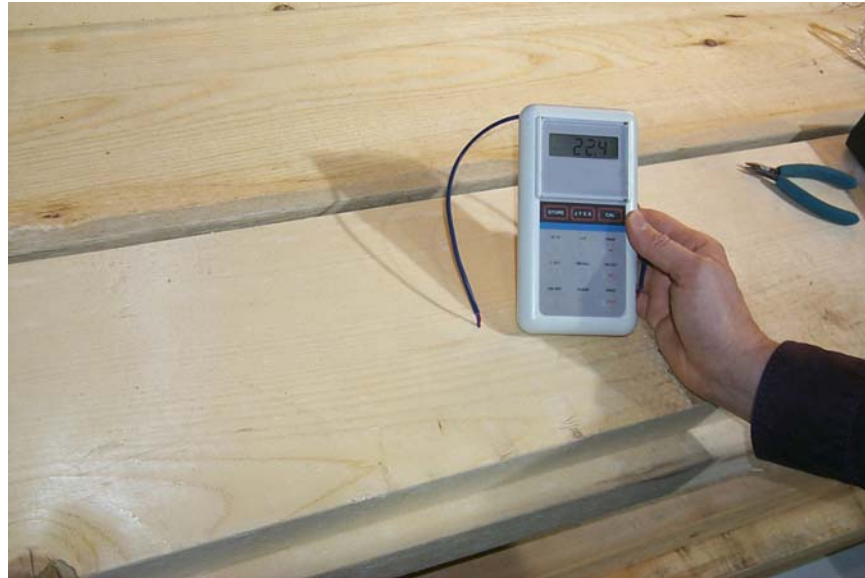
Figure 3: Hand-held digital thermometer fitted with thermocouple probe to measure internal wood temperature
