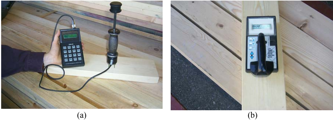
Figure 2: D.C. Resistance moisture meter (on left) and dielectric moisture meter (on right)
