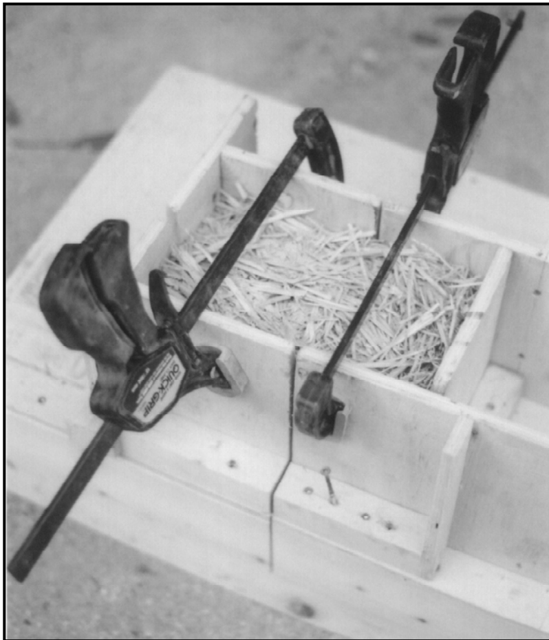
Fig. 3.4.3-1 The specimen cutting box
