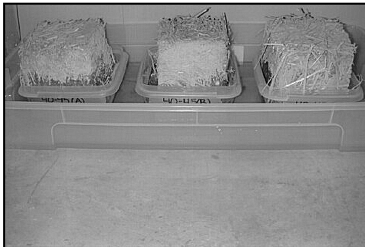
Fig. 7.2-1 Water uptake test set-up
