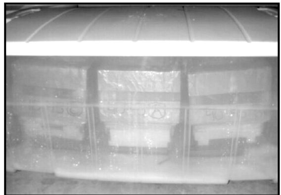
Fig. 5.2-5 Samples within 75% RH container
