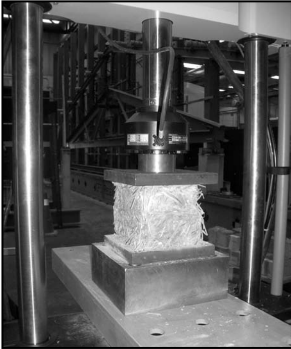
Fig 8.4-1 Typical compression (before)
