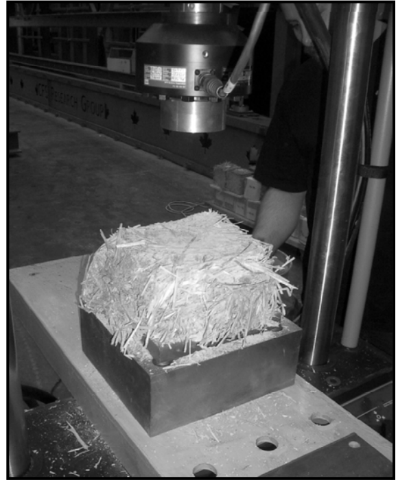
Fig. 8.4-2 Typical compression (after)
