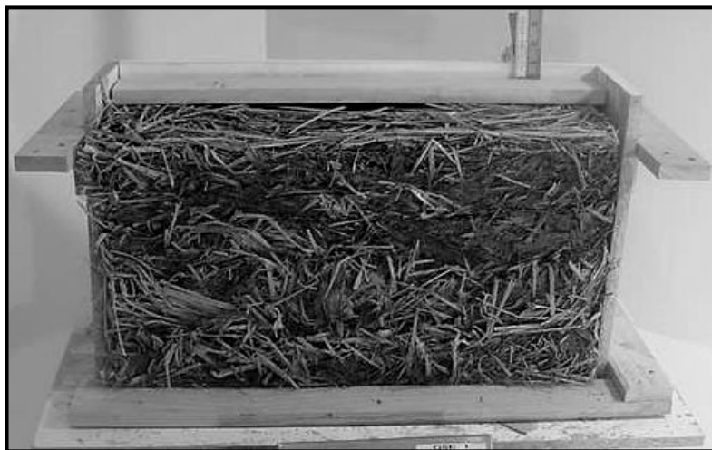
Fig. 9.2-1 Typical set-up for measuring settling.
