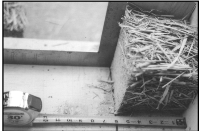
Fig. 3.4.3-5 Sample accuracy illustrated with square and tape
