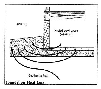
The most significant heat loss from a building foundation occurs in the perimeter band of soil immediately adjacent to the building. Heat loss at corners is most pronounced because it occurs in two directions.
