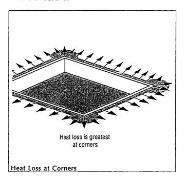
By strategically placing foundation insulation, this heat loss can be used to keep the footing from freezing and heaving.
