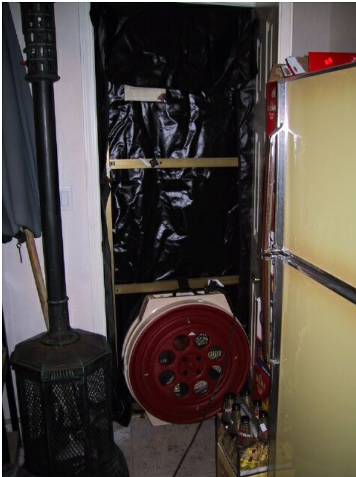
Figure 5: Fan Door Apparatus
