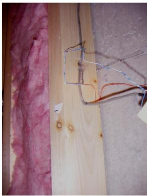
The upper portions of the stud were examined for mold or moisture accumulation evidence; none was seen (left hand test bay stud)
