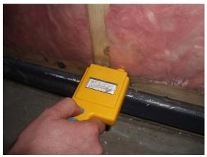
Moisture content measurements taken through the polyethylene ranged from "off scale high" (bottom plate) to 25% (1" up from bottom of stud) to 15% (corner of bottom plate): see complete list below.
