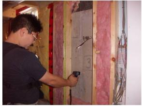
Measurement of concrete-insulation interface temperature with infrared laser thermometer
