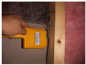
Delmhorst moisture meter measurements of the test bay stud, parallel to moisture content pins
