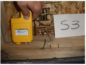
A gradient of moisture content measurements were taken across the width of the sill plates; measurements shown below.
