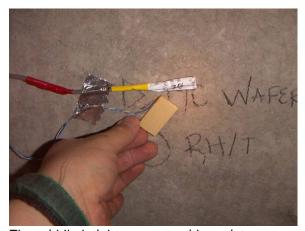
The middle-height concrete-side moisture wafer showed no mold evidence on the interior side.
