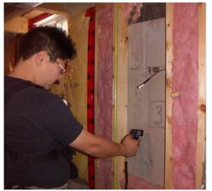
Figure 1.10: Vertical temperature gradient in frame-latex wall
