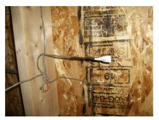
The relative humidity sensor in the south poly wall at mid-height (S3-RCNM) failed at the beginning of April, 2005. A replacement sensor was spliced in during the wall inspection.
