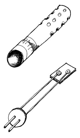
This sensor assembly was placed on the completed body of the housing after the housing was placed in the wall (to prevent the sensor from being pushed too far back into the unit and being exposed to the straw. The whole assembly is about 280mm (11") long, not counting the tails of the wire leads sticking out of the canister lid (100 to 150mm/4 to 6 inches). The moisture content in the wood block was recorded before being installed.
