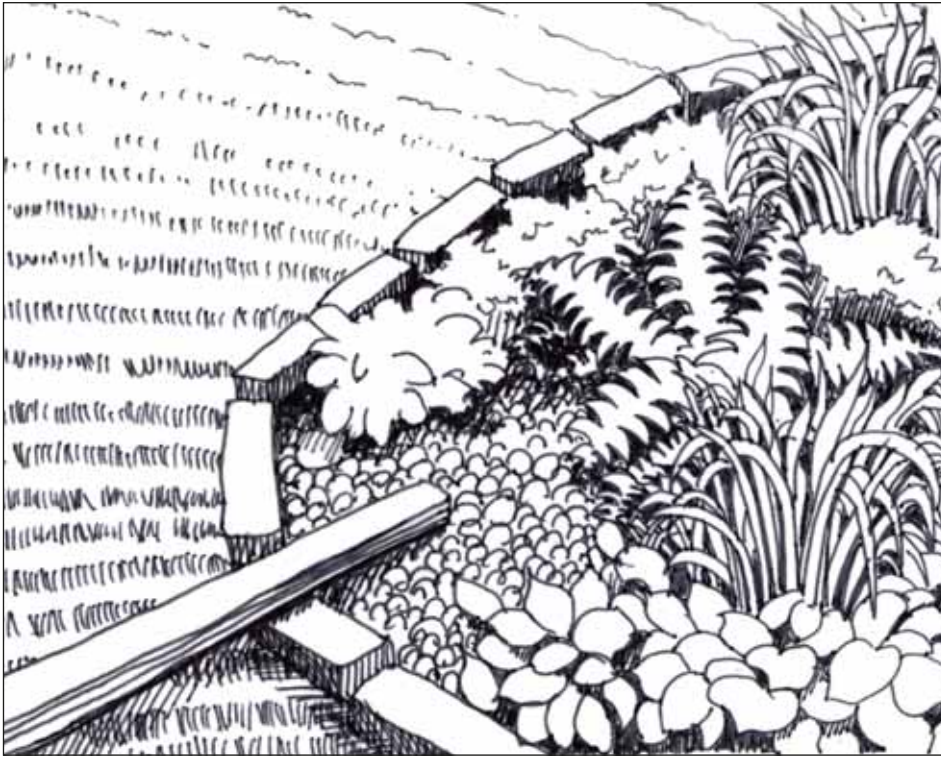
Figure 6 You can run a roof downspout extension directly into your rain garden. To prevent erosion, install a small bed of pebbles or a concrete splash pad under the end of the extension.
