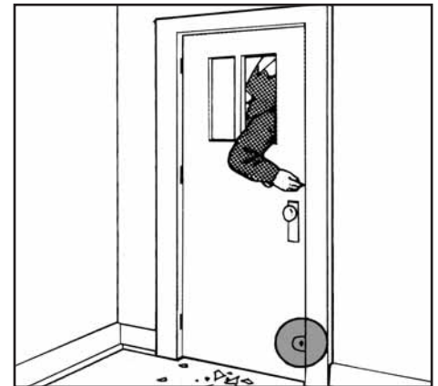
Figure 13 Breaking the glass will not help a burglar if the auxiliary lock is out of reach.
