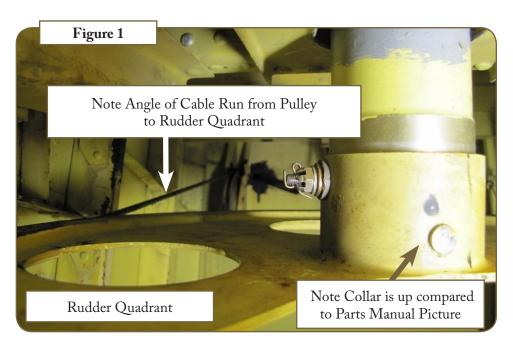
Also noted and seen in figure 3 was the quadrants misalignment of approximately 6.3 cm (2.5 in) away from the cable guard.
