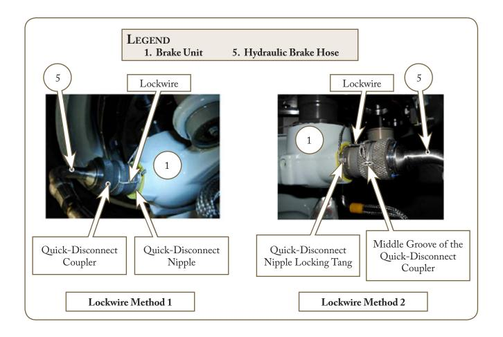
The following Bombardier Aircraft Maintenance Manual (AMM) Temporary Revisions (TR) were released May 2011 which have introduced instructions to utilize 2 methods of lock wire on the brake QD for the CRJ705/900/1000. The addition of the lock wire is to prevent the inadvertent unlocking of the QD.
