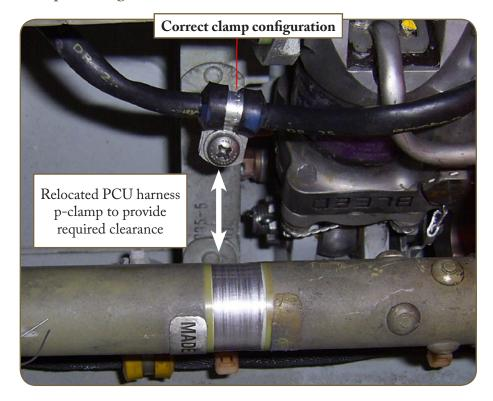
Presently in the AMM, there is no mention of the required p-clamp positioning that secures the wiring harnesses of the PCU's.
