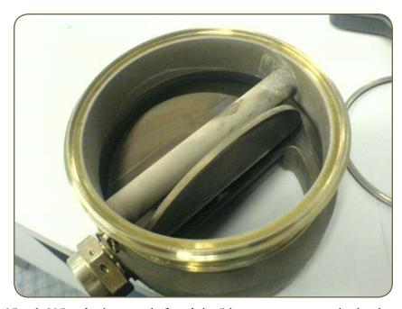
Maintenance personnel accomplished FIM 71-05 task 805 and subsequently found the 5th stage compressor check valve stuck open. The valve was replaced as the corrective action and the aeroplane was returned to service.
