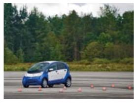
In addition to testing the vehicles at various temperatures in laboratories, eTV used test facilities in Vancouver to evaluate the i-MiEV's performance in temperatures as low as -20 degrees Celsius.
