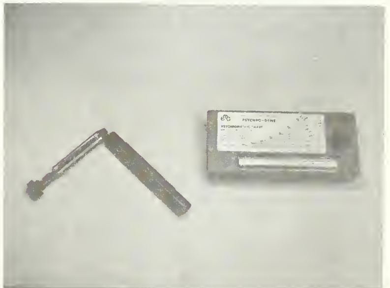
Fig. 30 Sling psychrometer (left) and dry bulb – wet bulb meter (a small fan blows air over the wet and dry bulbs).
