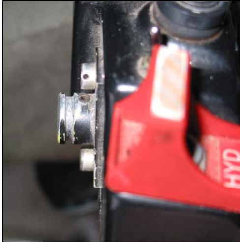
Photo 3. Collective locking button showing groove wear
