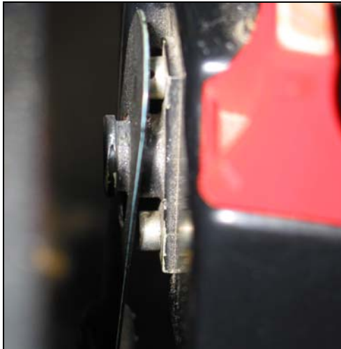
Photo 4. Collective locking plate improperly engaged on shoulder of button, not groove (accident helicopter)
