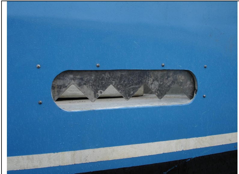
Photo 5. Saw tooth style freeing port viewed from outside vessel
