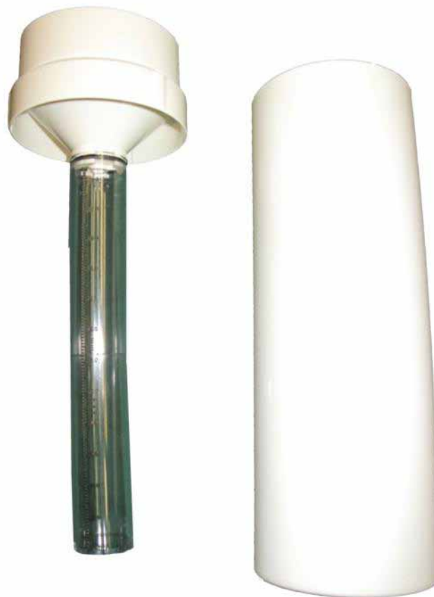
Figure 2-1: Rain gauge – type-B (collector, funnel and graduate)
