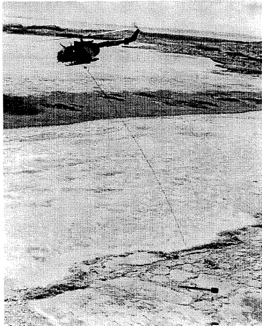
Figure 1.0.1: EIS sensor bird being towed by a Canadian Coast Guard helicopter.
