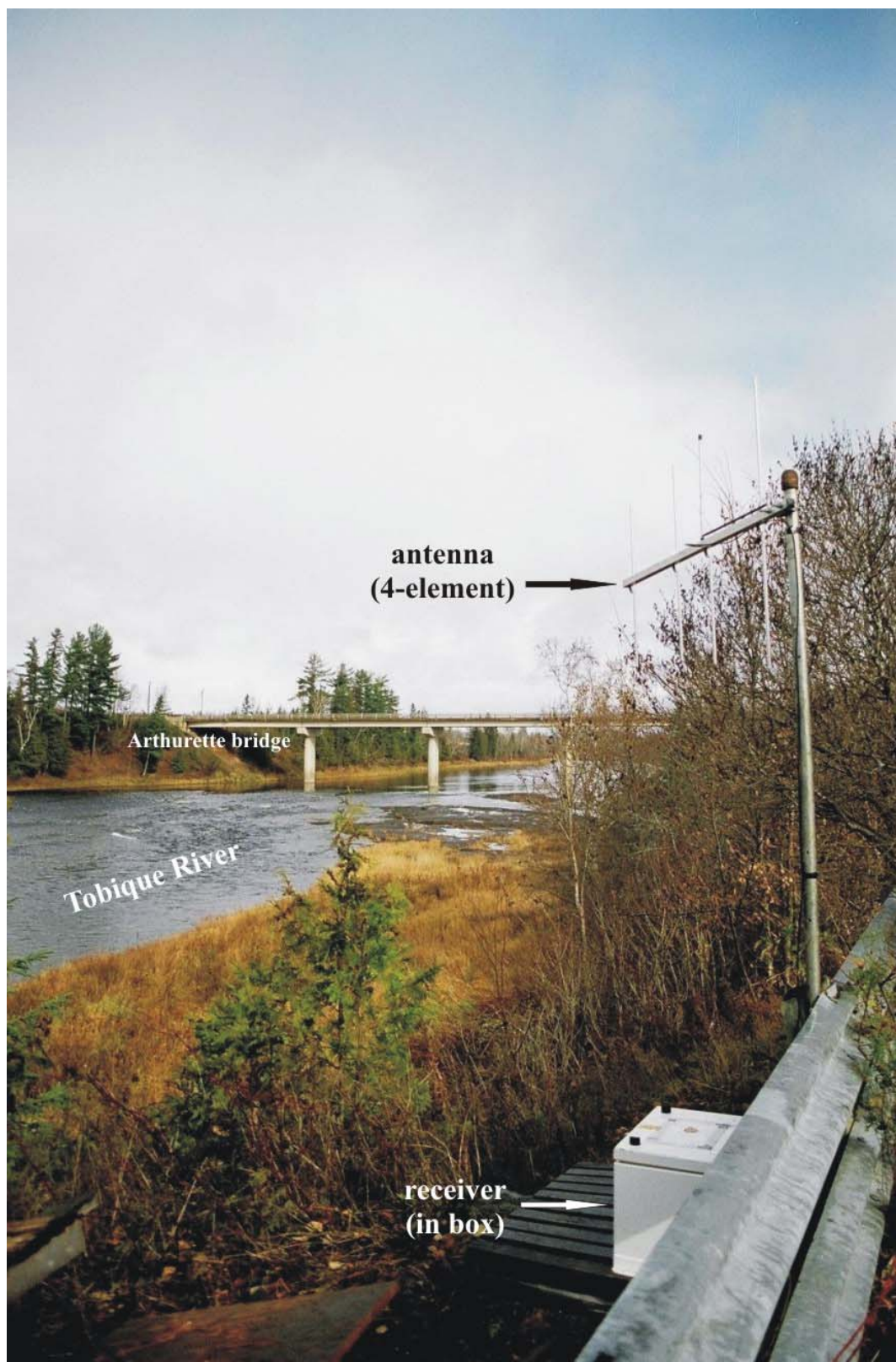
Figure 5. Photo showing typical installation of antenna connected to receiver (Arthurette location).
