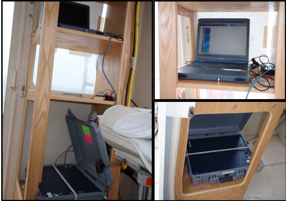
Figure 2: Left – Custom hardwood shelf on back wheelhouse wall. BioSonics data acquisition computer on top shelf; with BioSonics DT-X digital echosounder surface unit below. The white object in the foreground is a passenger seat (folded down). Right Top – BioSonics computer with blue Ethernet cable leading to the DT-X surface unit. Right Bottom – BioSonics DT-X digital echosounder surface unit strapped in place.
