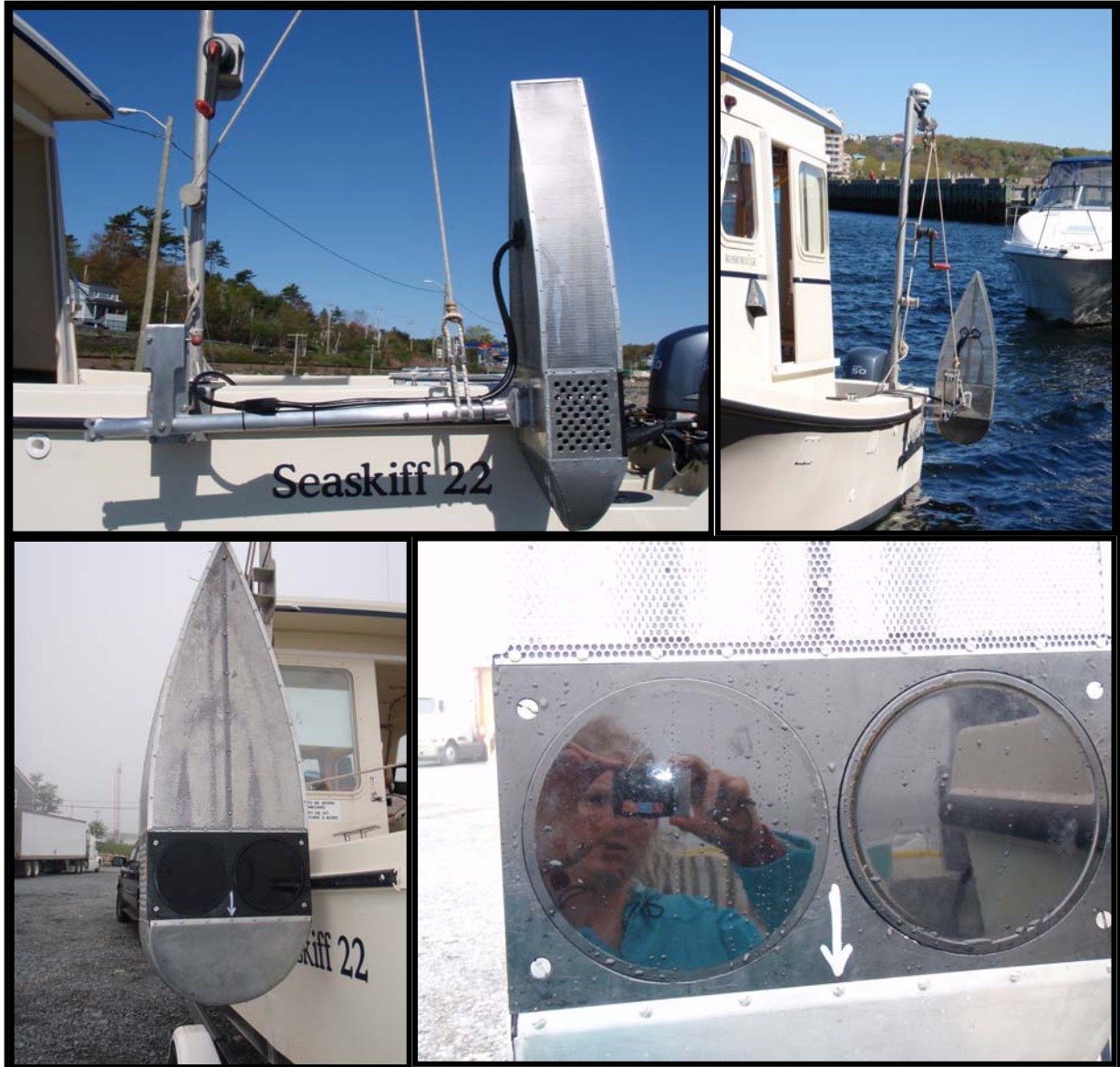
Figure 4: Transducer cage raised for transport. Note tapered tail section which is 'see through' due to its construction from perforated aircraft aluminum. Blunt nose constructed of solid sheet aluminum. The paint can sized transducers are bolted inside the cage below its support arm in a sturdy aluminum frame (large perforations on its side). On the bottom of the cage, black plastic faring surrounds the black circular transducer surfaces, which have a mirror like smoothness.
