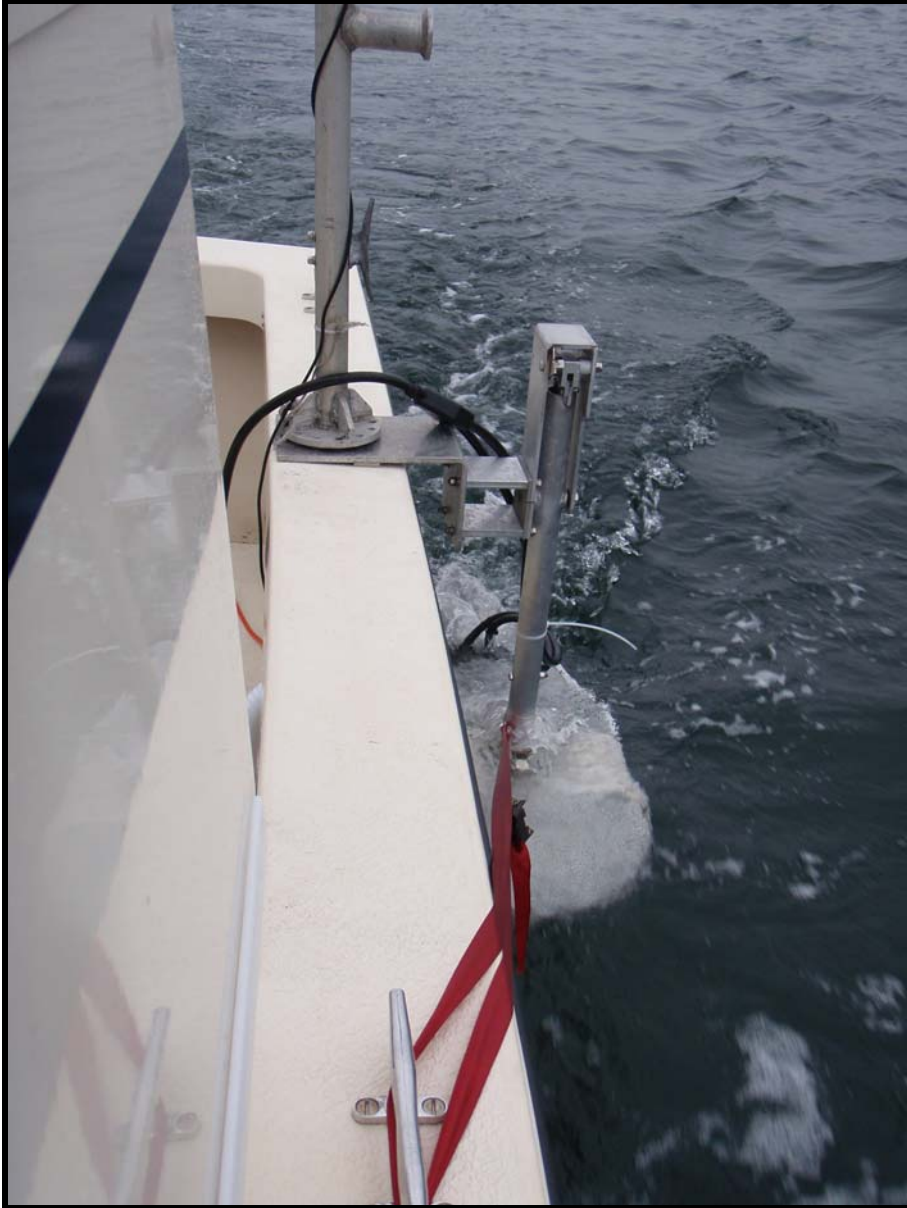
Figure 6: Transducer cage in place while running a survey. A red ratchet strap holds the bottom of the cage support arm in position, preventing the water pressure at 4 knots from popping the support arm latch (device at the top of the arm). The top of the cage is just below the water surface. Note how the blunt nose of the cage creates a small standing wave which then falls into the perforated tail section. This creates a very smooth flow of water around the cage, and laminar flow over the transducer surfaces.
