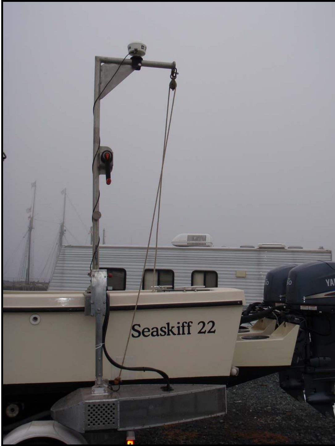
Figure 5: Cage in survey position. Note alignment of cage support arm with davit post, and dGPS antenna on top of davit (i.e. almost directly above the transducers). Bottom of cage is higher than vessel keel, providing added protection in case of grounding. Cage support rope is removed from block during surveys.
