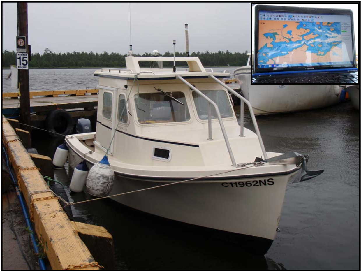
Figure 1: 22' twin engine Cape Sable style research vessel with enclosed wheelhouse. Insert - Navigation notebook computer at helm running Nobeltec, Inc. VNS™ Max Pro navigation software.
