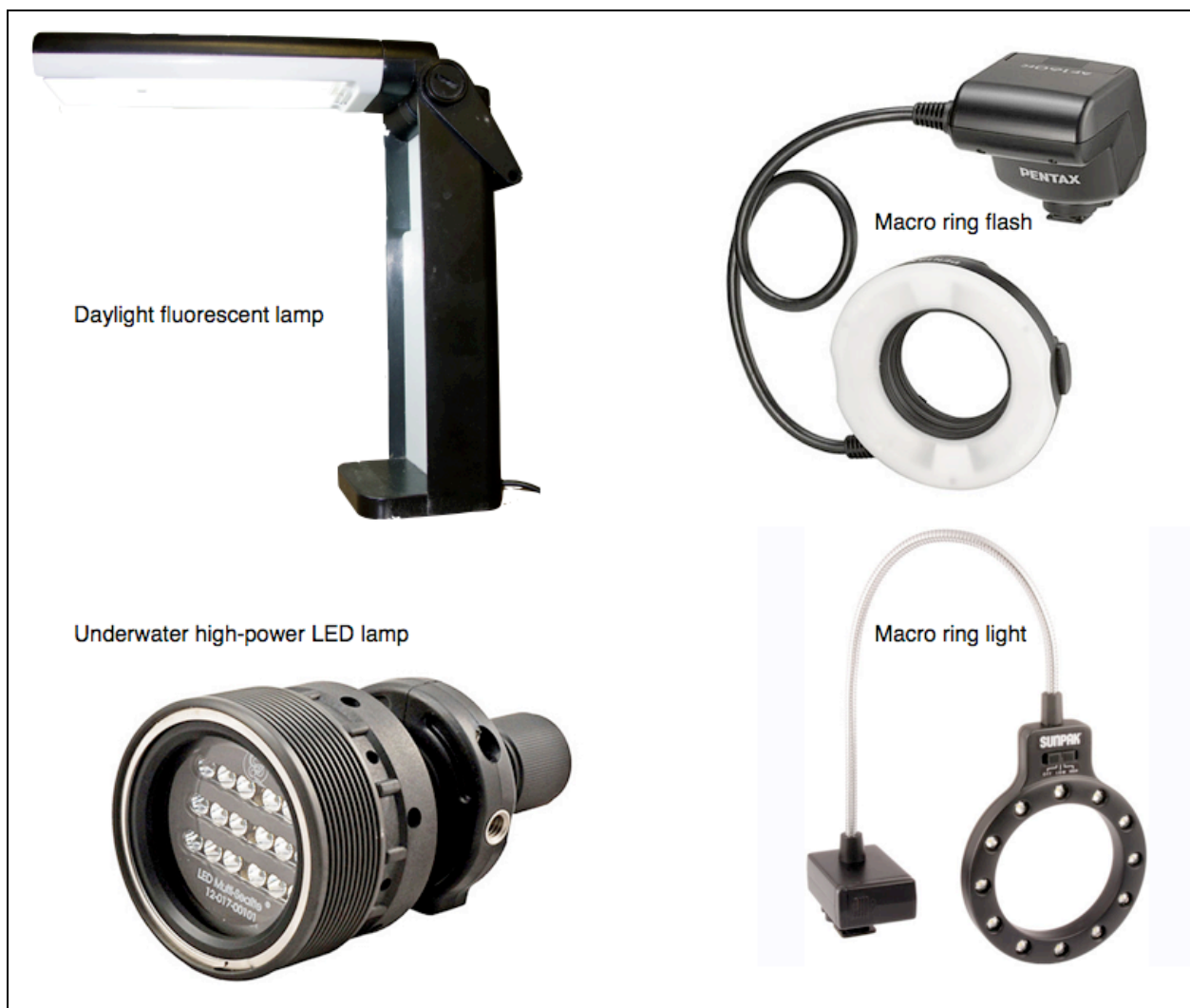
Figure 26. Examples of light sources for field and lab work. Many now use LEDs for energy-efficiency (portability with battery packs) and lower heat output.
