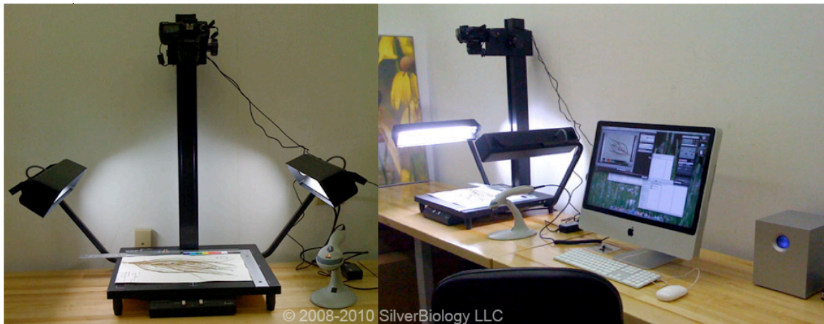
Figure 51. Setup for high-volume digitization of collection materials with SilverImage .
