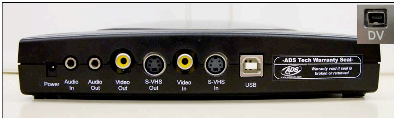
Figure 54. Video-to-DVD converter box. Ports include S-Video (round with pinholes) and RCA composite (yellow). FireWire400 is available by a mini-port in front (inset; "DV"). Output to computer is by USB2.
