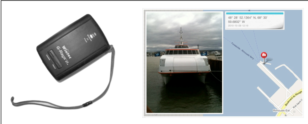
Figure 32. Geologging tools. Left, a bluetooth GPS data logger for recording tracks Right, a smartphone app exporting an image as a mapcard (a photo on map).
