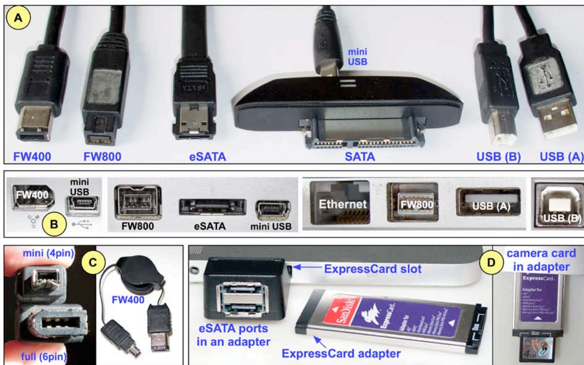
Figure 36. Examples of data ports. (A) Cable plugs: FW400, FW800, eSATA, SATA, USB (square and flat). (B) Cable ports. (C) Mini (video) and full-size (computer) plugs. (D) ExpressCard slot and adapter in a laptop computer.
