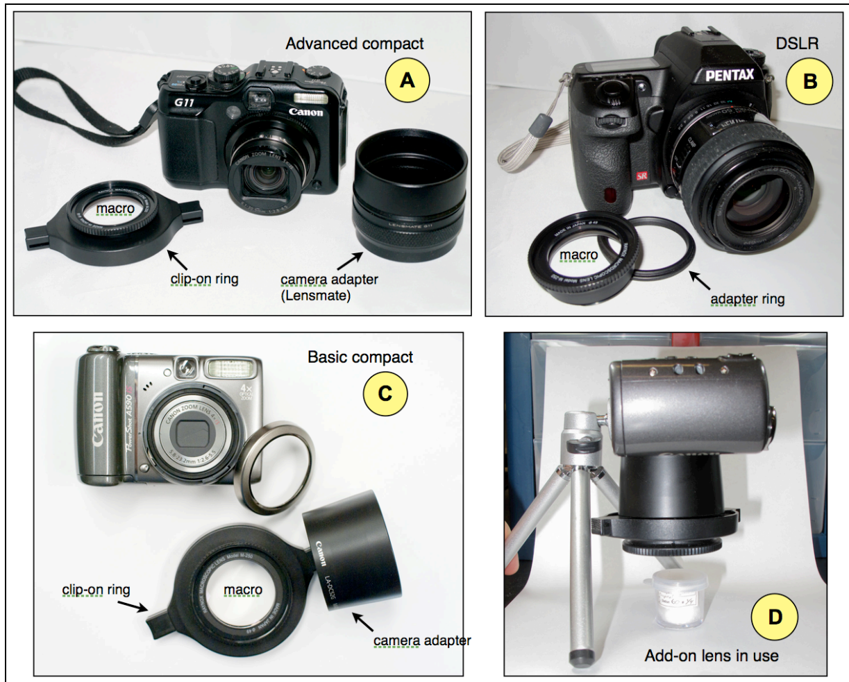
Figure 28. Example of a magnifying add-on lens: Raynox DCR-250 being used on (A) an advanced compact camera with set of Lensmate adapters; (B) a DSLR camera with a 43–49 mm filter adapter ring; (C) a basic compact camera with adapters, (D) here seen assembled for use.
